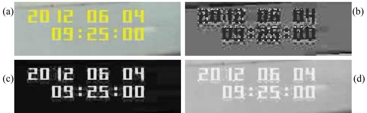
Figure 4.4: (a) Original image, (b) Hue component (c) Saturation component (d) Value component
