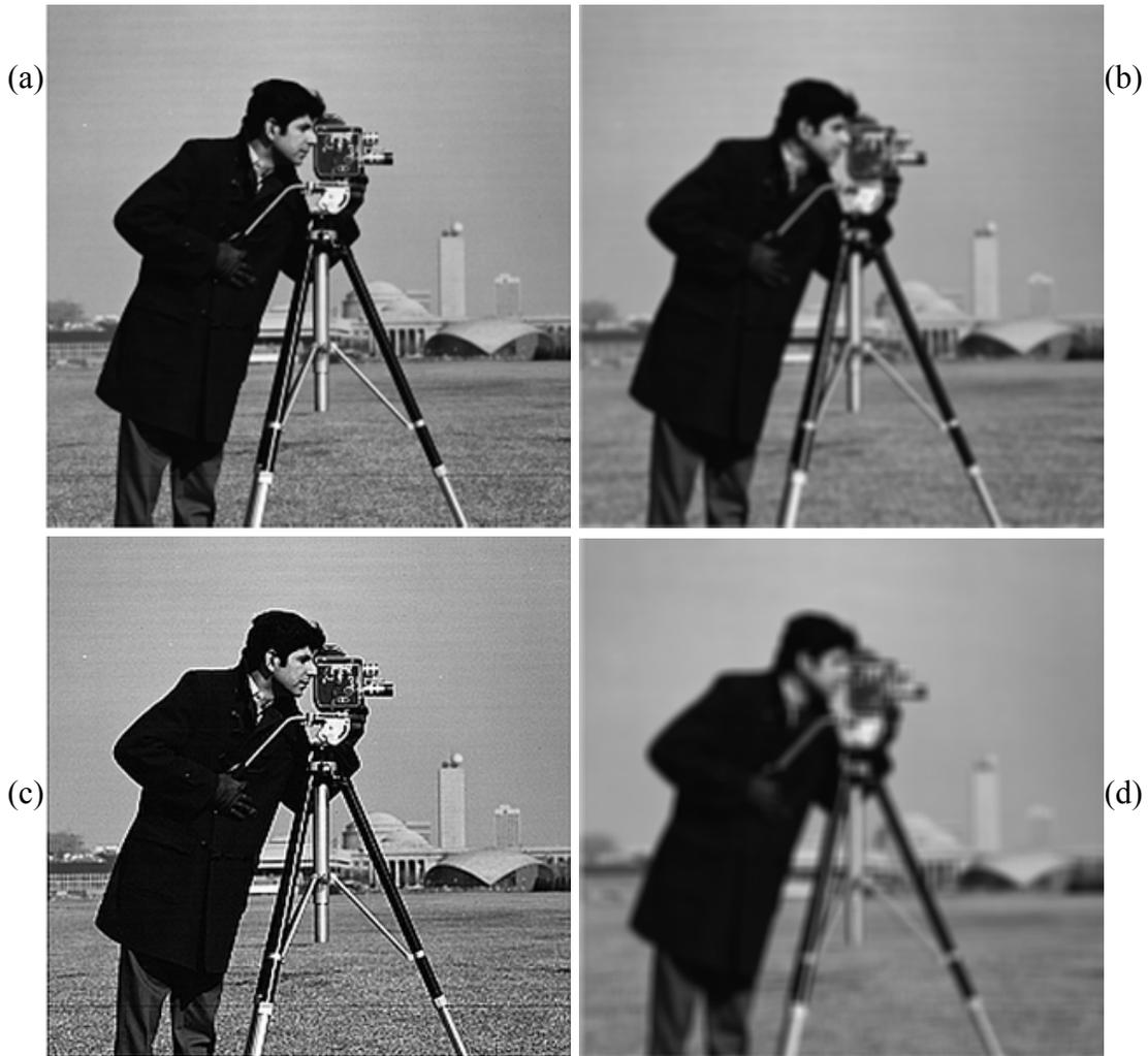
Figure 3.2: Applying different filters to an image (a) Original image [MathWorks Inc. 2011] (b) Smoothing filter (c) Sharpening filter (d) Gaussian
