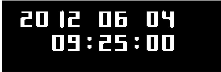
Figure 4.5: Enlarged timestamp binary image after applying threshold
